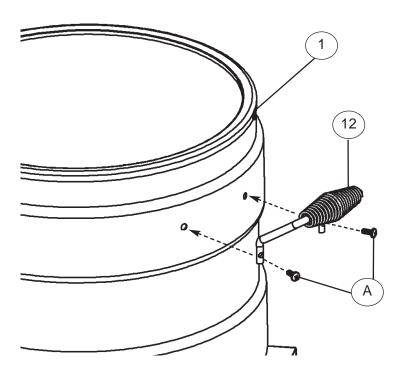
Secure side handles (12) to outer shell (1) using pan head screws (A).
